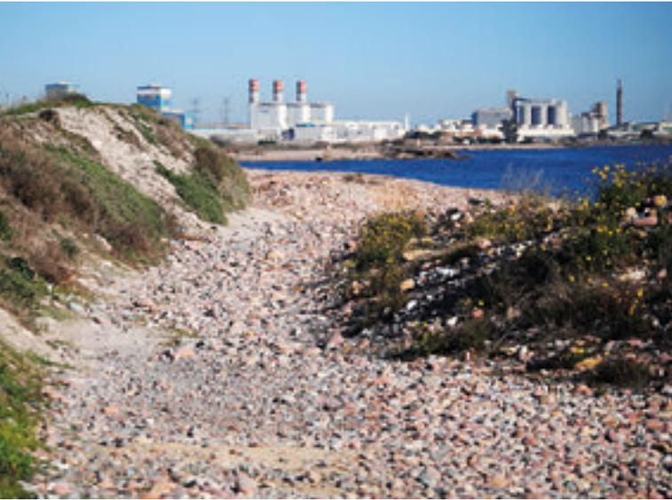
Effects of coastal erosion on the dunes at La Marjal dels Moros (Sagunto), where the increasing force of storms in recent years has added to the effect of the lengthening of the breakwaters at the Sagunto port. The old access path, around 3 metres wide, and the dune platform separating it from the sea – around 30 metres wide – have disappeared in the last few years. In the central photograph, the remaining dune community of *Juniperus macrocarpa* in Prat de Cabanes-Torreblanca.
