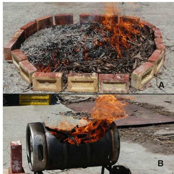
FIGURE 1. Ash produced under controlled conditions a) low intensity fire b) high intensity fire.
